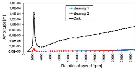
Fig. 6. Vibration amplitudes of the bearing journals and of the disk (variant no. 1).
