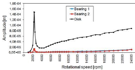
Fig. 12. Vibration amplitudes of the bearing journals and of the disk (variant no. 4).
