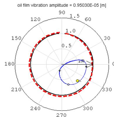
Fig. 16. Vibration trajectory of the foil bearing's journal at 2,350 rpm (variant no. 1).
