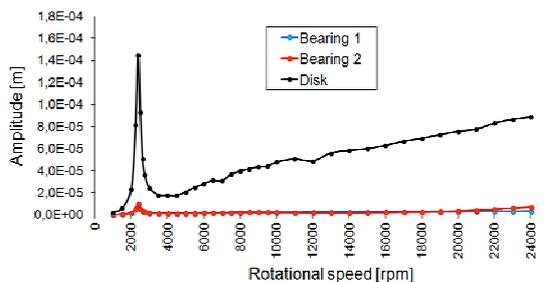
Fig. 14. Vibration amplitudes of the bearing journals and of the disk (variant no. 5).
