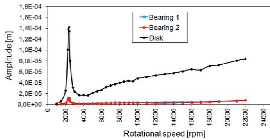
Fig. 10. Vibration amplitudes of the bearing journals and of the disk (variant no. 3).
