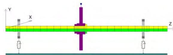
Fig. 2. The numerical model of the rotor.
