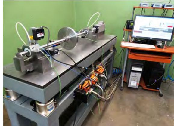
Fig. 1. Test rig with a flexible rotor and two slide bearings.
