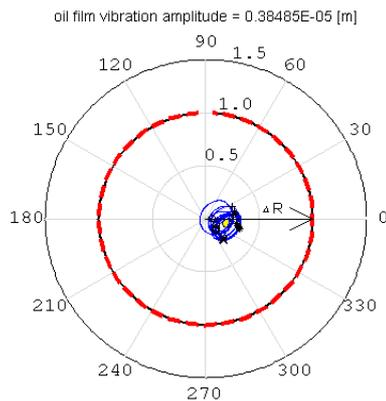
Fig. 17. Vibration trajectory of the foil bearing's journal at 22,000 rpm (variant no. 1).
