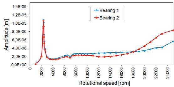
Fig. 7. Vibration amplitudes of the bearing journals (variant no. 1).
