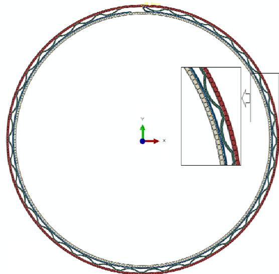
Fig. 3. FEM model of the foil bearing structure with one bump foil (variant no. 1).
