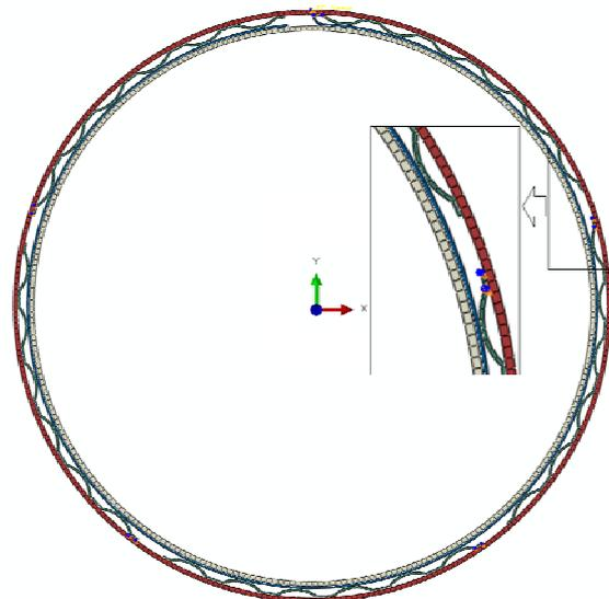
Fig. 4. FEM model of the foil bearing structure with five bump foils (variant no. 3).
